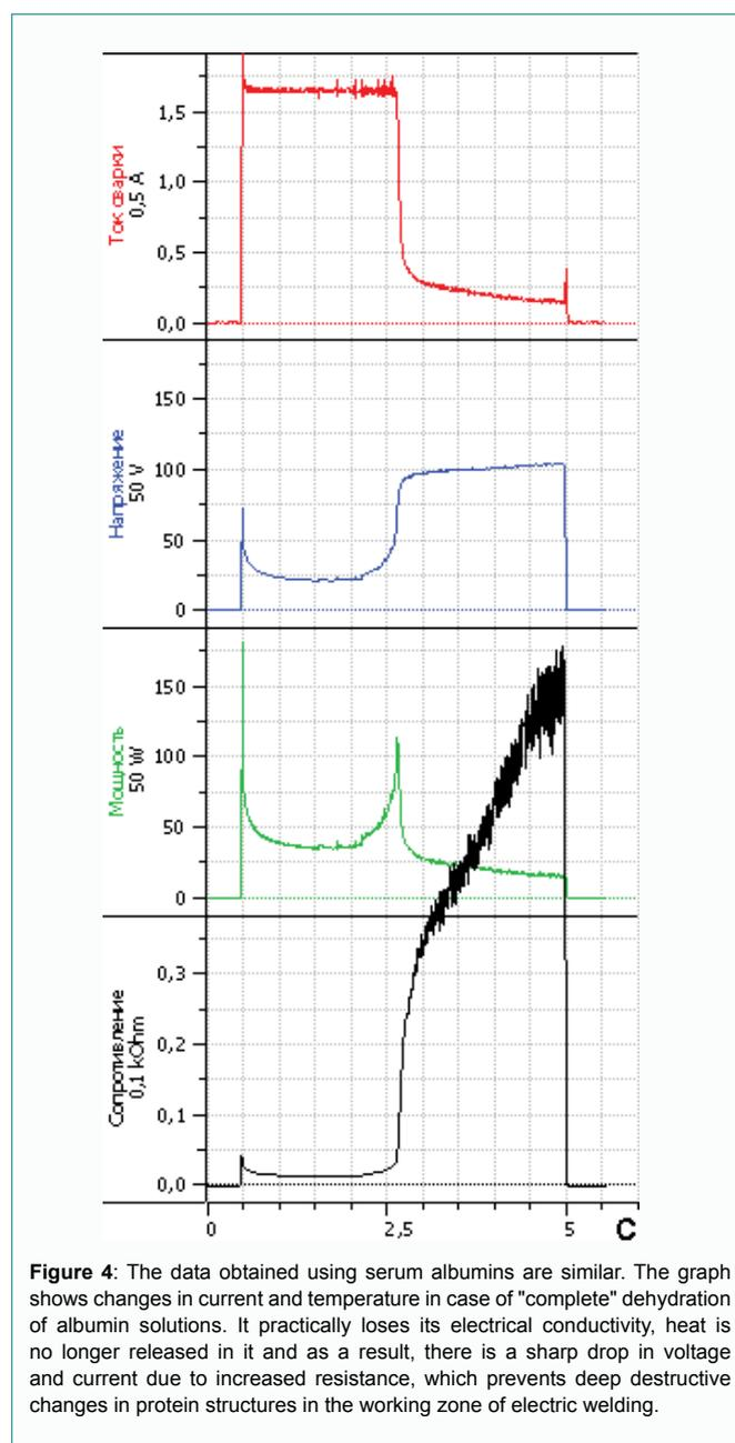
**Figure 4:** The data obtained using serum albumins are similar. The graph shows changes in current and temperature in case of "complete" dehydration of albumin solutions. It practically loses its electrical conductivity, heat is no longer released in it and as a result, there is a sharp drop in voltage and current due to increased resistance, which prevents deep destructive changes in protein structures in the working zone of electric welding.
