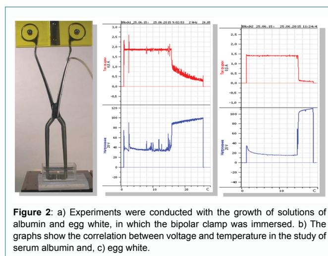
**Figure 2:** a) Experiments were conducted with the growth of solutions of albumin and egg white, in which the bipolar clamp was immersed. b) The graphs show the correlation between voltage and temperature in the study of serum albumin and, c) egg white.
