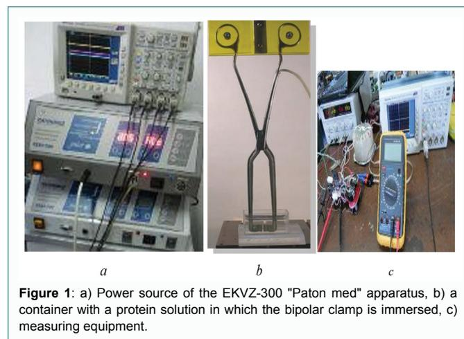
**Figure 1:** a) Power source of the EKVZ-300 "Paton med" apparatus, b) a container with a protein solution in which the bipolar clamp is immersed, c) measuring equipment.
