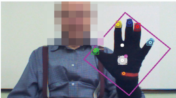
Figure 1A: System setup for the near mode (upper limb tasks). Colored gloves are used for the tracking and for computer interactions (for example to select actions by moving and closing the hand on drawn squares). Position of hand 3D centroid (solid white point); colored markers on glove; hand 3D bounding box with centroid (solid magenta line and point).
