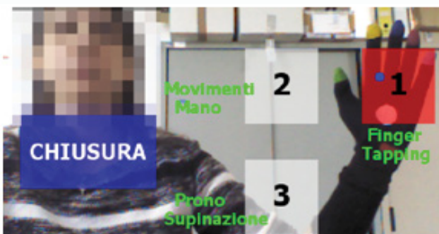
Figure 1B: Example of HCI for upper limb task selection: exercise is selected by moving the hand on interactive objects (object color changes from white to red) and closing the hand to confirm the choice.
