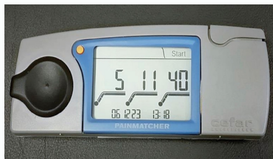
Figure 2: The Pain Matcher (Cefar Medical AB, Sweden) is an instrument for electrical stimulation that provides constant current stimulation despite variable skin resistance. The electrical charge per second is extremely low and causes no tissue damage. The intensity value (0 to 99) is directly related to the pulse width and is displayed on a liquid crystal screen.
