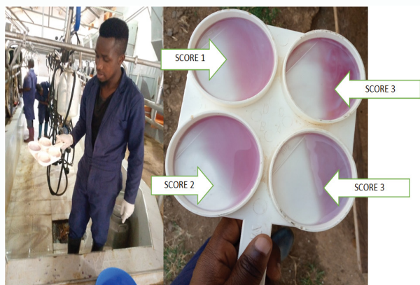
Figure 3: Reaction of milk with CMT reagent.
