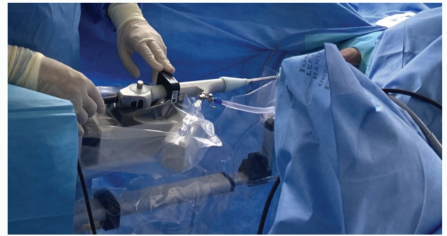
Figure 2: Fixation of the flexible ureterscope in the manipulator of the avicenna roboflex.
